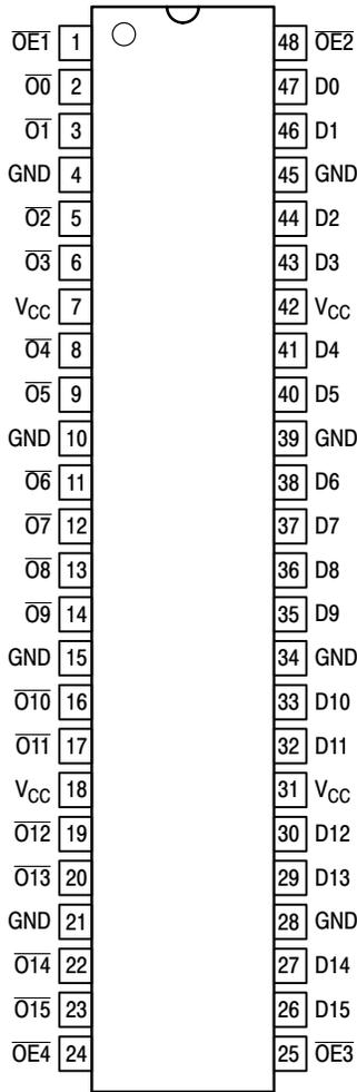
**Figure 1. 48-Lead Pinout**
