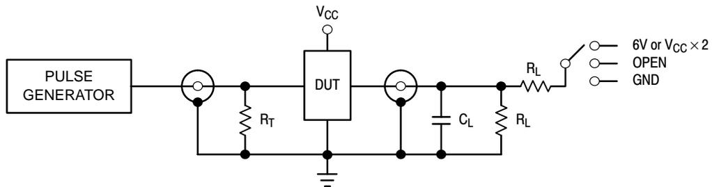
**Figure 7. Test Circuit**
