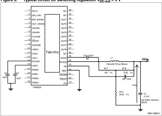
Figure 9. Typical circuit for switching regulation  $V_{DC-out} = 5 V$
