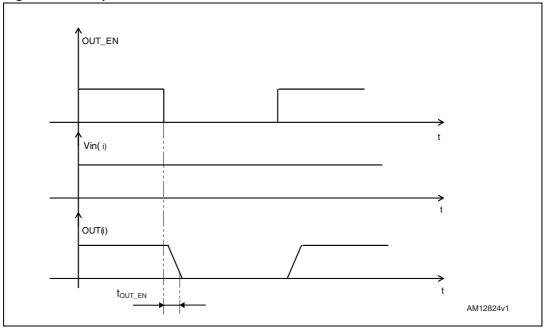
Figure 4. Output channel enable/disable behavior
