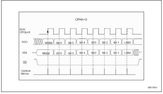
Figure 3. SPI mode diagram
