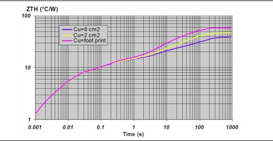
Figure 11. PSSO36 thermal impedance vs. time
