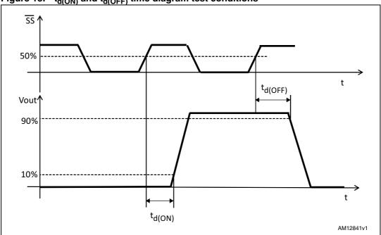
Figure 15.  $t_{d(ON)}$  and  $t_{d(OFF)}$  time diagram test conditions
