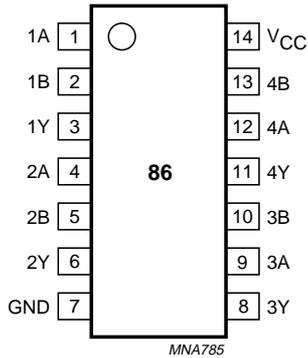
Fig.1 Pin configuration SO14 and (T)SSOP14.
