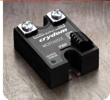
The MCST, MCSP and MCSS series of controls is designed to provide adjustable surge reducing soft-start and soft-stop control for any load which would benefit from a gradual application or shutdown of power, and provide Crydom SSR switching within one package.
