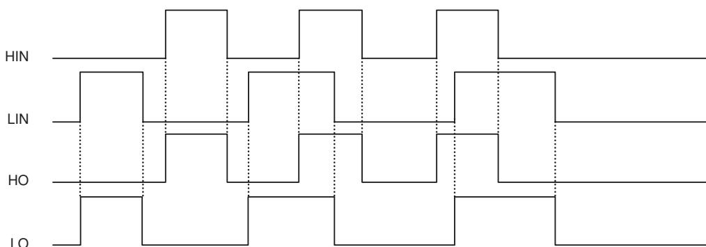
**2. Vcc2com (VBS) Supply Under Voltage Lockout Timing Diagram**
