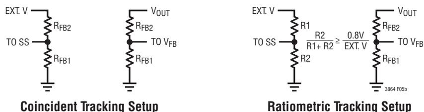
Figure 5(b): Setup for Ratiometric and Coincident Tracking
