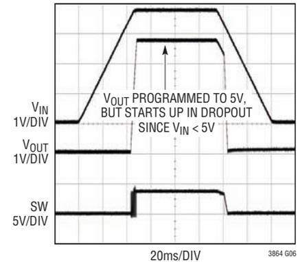
$V_{IN} = 0\text{V}$  TO 3.8V THEN BACK TO 0V
