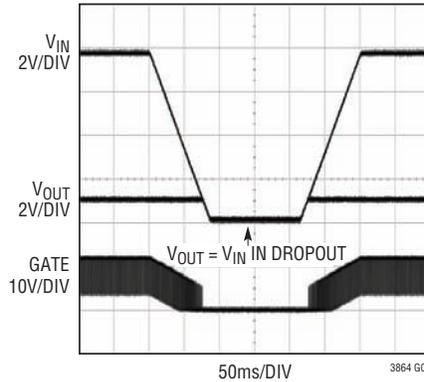
$V_{IN}$  TRANSIENT: 12V TO 4V AND BACK TO 12V
