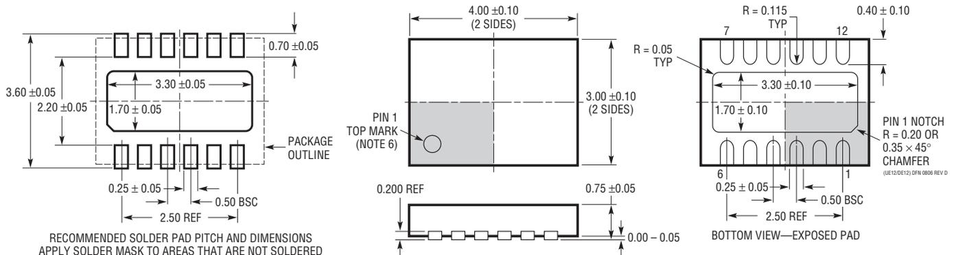
RECOMMENDED SOLDER PAD PITCH AND DIMENSIONS APPLY SOLDER MASK TO AREAS THAT ARE NOT SOLDERED
