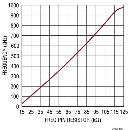
Figure 2. Switching Frequency vs Resistor on FREQ
