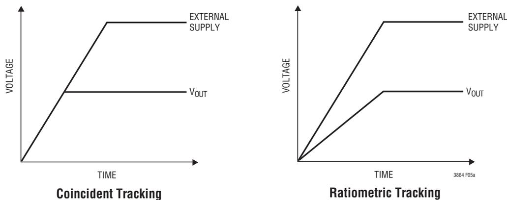
Figure 5(a). Two Different Modes of Output Tracking
