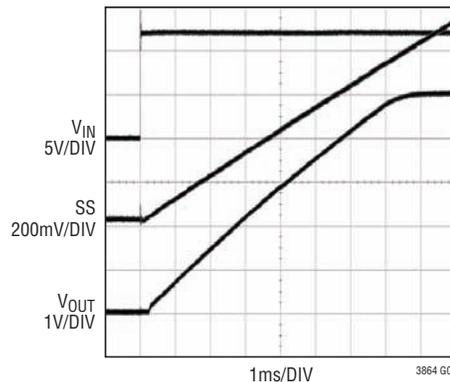
$V_{IN} = 12\text{V}$ ,  $V_{OUT} = 5\text{V}$
