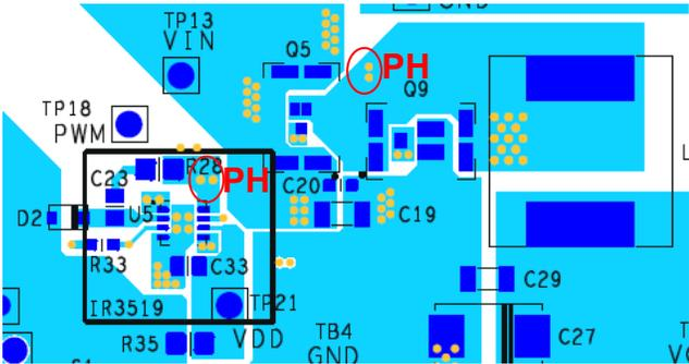
Figure 1: Phase Node Sense with Less Noise
