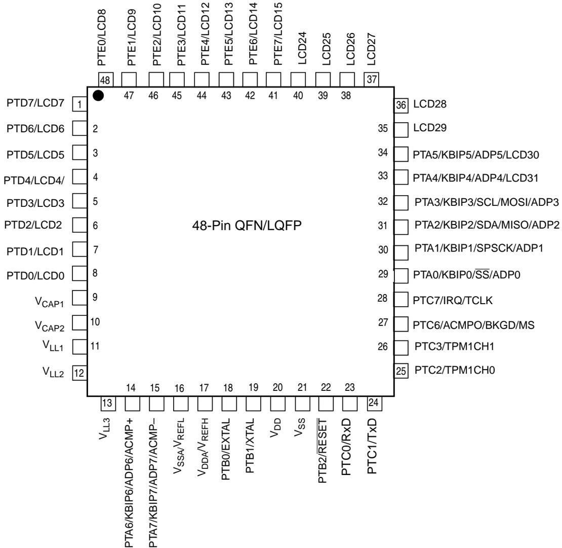
Note: V<sub>REFH</sub>/V<sub>REFL</sub> are internally connected to V<sub>DDA</sub>/V<sub>SSA</sub>
