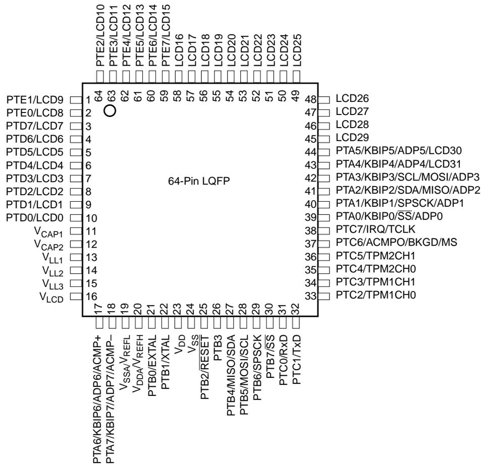
Note:  $V_{REFH}/V_{REFL}$  are internally connected to  $V_{DDA}/V_{SSA}$ .
