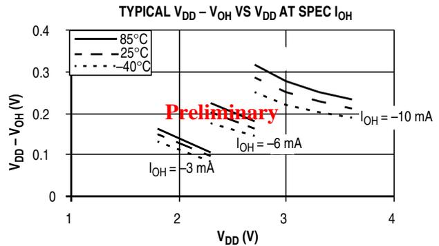
Table 17. Typical High-Side (Source) Characteristics (LCD/GPIO pins) — High Drive (PTxDSn = 1)
