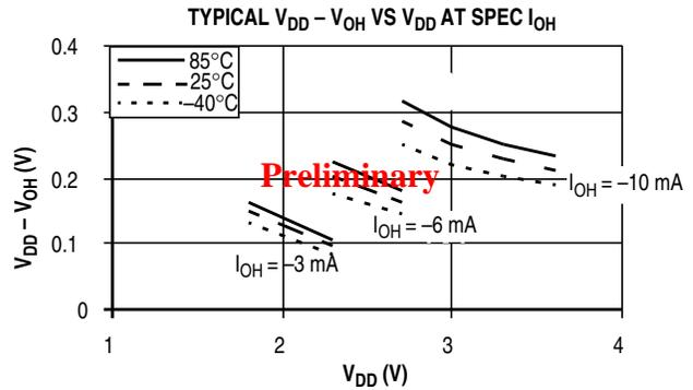
Table 13. Typical High-Side (Source) Characteristics(Non LCD pins) — High Drive (PTxDSn = 1)
