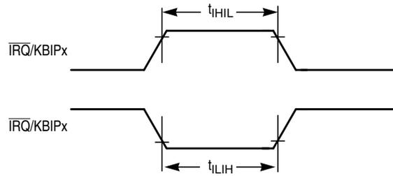
Figure 10.  $\overline{\text{IRQ}}/\text{KBIPx}$  Timing
