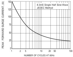
FIG.5 MAXIMUM NON-REPETITIVE FORWARD SURGE CURRENT
