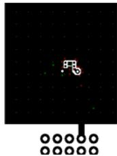
c. 95 °C/W when mounted on a 1 in<sup>2</sup> pad of 2 oz copper.
