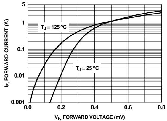
**Figure 12. Schottky Diode Forward Voltage**
