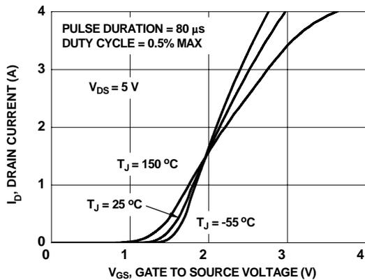
Figure 5. Transfer Characteristics
