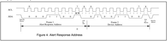
The F75393 provides SMBus address option function. Pull high register (Alert Pin) to select SMBus address by power on strapping and entry key writing. These two conditions must be done both for address selection. If you only option pull high register without
