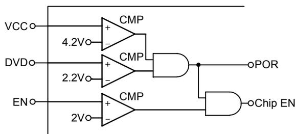
Figure 1. Power Ready (POR) Detection
