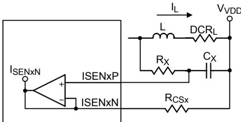
Figure 12. VDD Controller : Lossless Inductor Sensing
