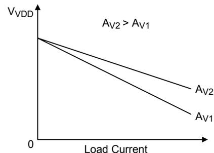
Figure 9. VDD Controller : Error Amplifier gain (AV) Influence on V<sub>VDD</sub> Accuracy
