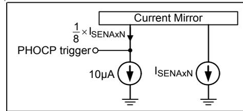
Figure 13. VDD Controller : Per-Phase OCP Setting
