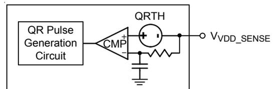
Figure 14. VDD Controller : Quick Response Triggering Circuit
