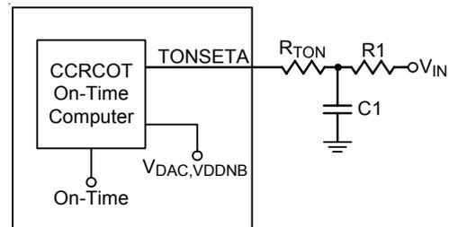
Figure 18. VDDNB Controller : On-Time Setting with R<sub>C</sub> Filter
