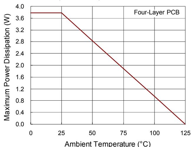
Figure 22. Derating Curve of Maximum Power Dissipation
