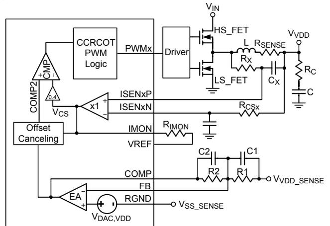
Figure 8. VDD Controller : Simplified Schematic for Droop and Remote Sense in CCM
