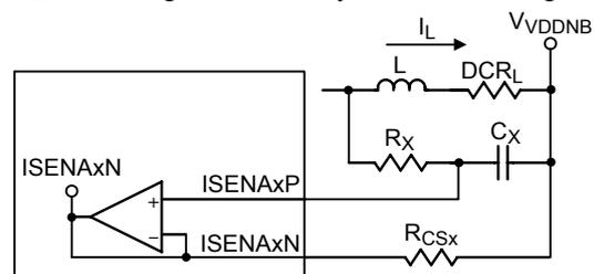
Figure 19. VDDNB Controller : Lossless Inductor Sensing
