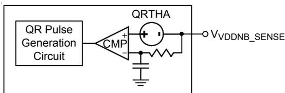
Figure 21. VDDNB Controller : Quick Response Triggering Circuit
