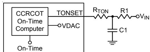
Figure 11. VDD Controller : On-Time Setting with R<sub>C</sub> filter
