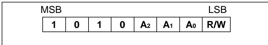
Figure 7 · Device Address
