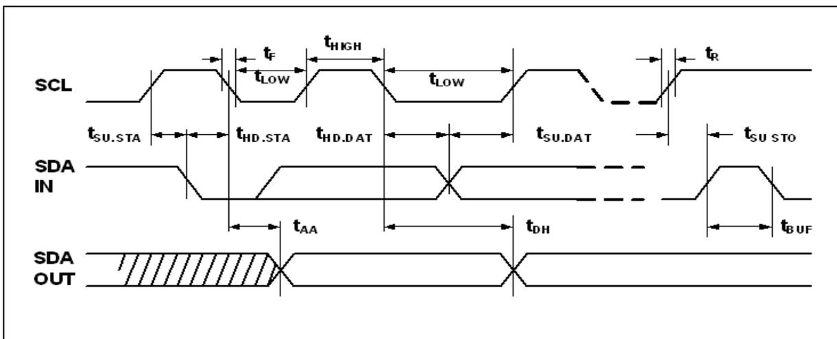
Figure 2 · SCL: Serial Clock, SDA: Serial Data I/O
