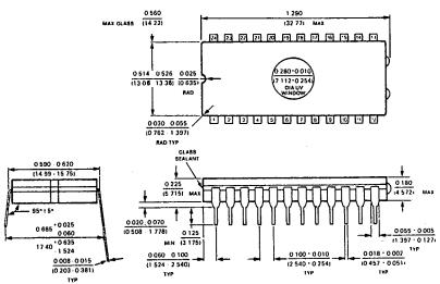
UV Window Cavity Dual-In-Line Package (Q)
