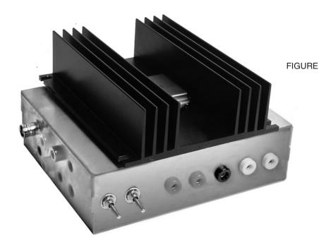
FIGURE 2. EXTERNAL WITH HEATSINK (HEAT-SINK, AMPLIFIER, CONNECTOR'S AND SWITCHES NOT SUPPLIED).
