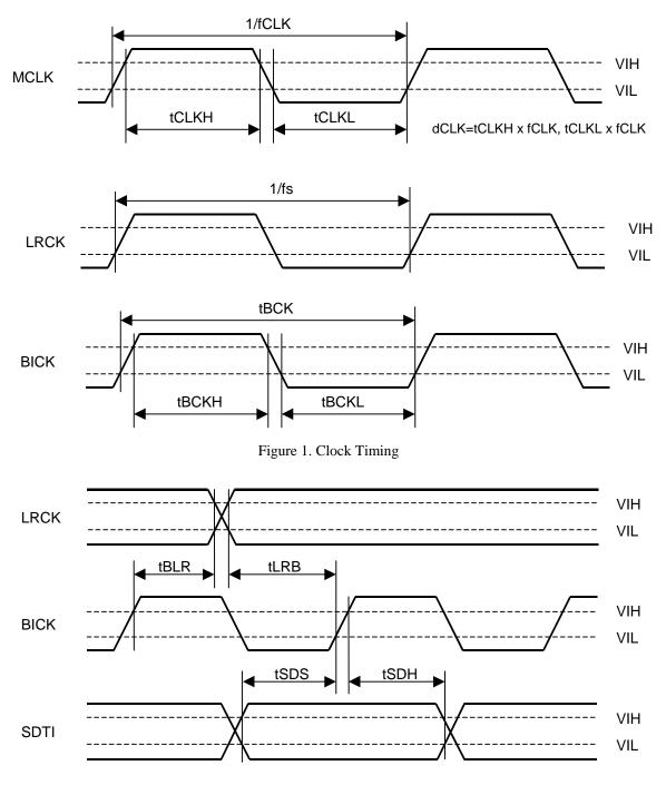
Figure 2. Serial Interface Timing
