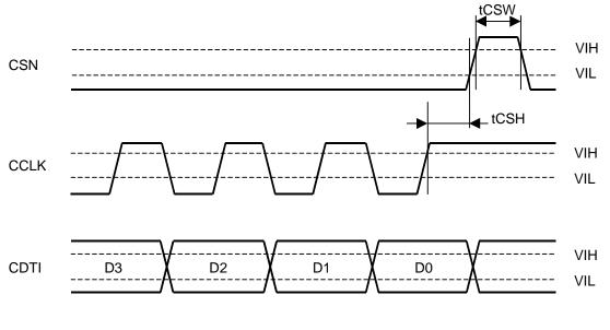
Figure 4. WRITE Data Input Timing
