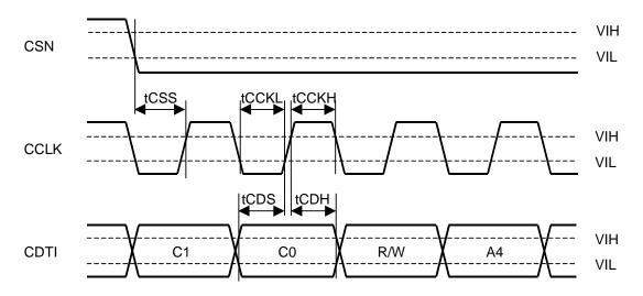
Figure 3. WRITE Command Input Timing
