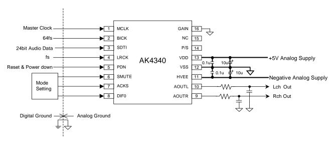
Figure 15. Typical Connection Diagram (Parallel Control Mode, GAIN=0dB)
