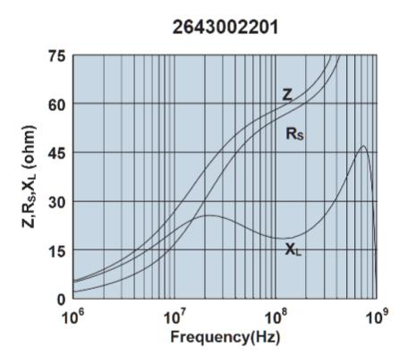
Impedance, reactance, and resistance vs. frequency.
