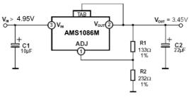
$$V_{OUT} = V_{REF} \times \left(1 + \frac{R2}{R1}\right) + I_{ADJ} \times R2$$
