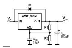
Internal resistors are limiting the internal current paths on the AMS1086M adjustment pin, therefore even with capacitors on the adjustment pin no protection diode is needed to ensure device safety under short-circuit conditions.
