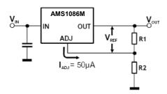
This current is normally the specified minimum load current of 7mA. Because  $I_{\text{ADJ}}$  is very small and constant it represents a small error and it can usually be ignored.
