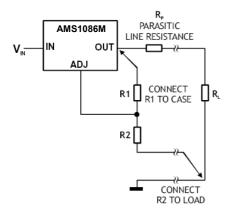
The best load regulation is obtained when the top of the resistor divider R1 is connected directly to the case not to the load. If R1 were connected to the load, the effective resistance between the regulator and the load would be:
