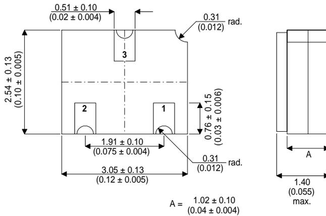
**Bipolar NPN Device in a Hermetically sealed LCC1 Ceramic Surface Mount Package for High Reliability Applications**
