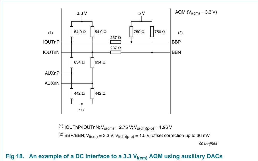
Fig 18. An example of a DC interface to a 3.3  $V_{i(cm)}$  AQM using auxiliary DACs
