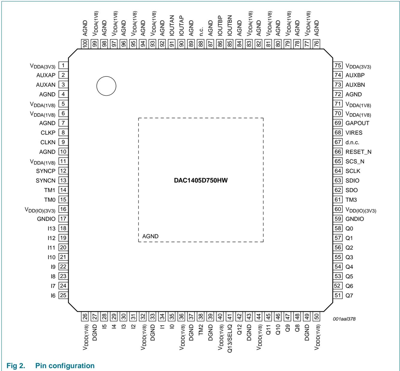
**Fig 2. Pin configuration**
