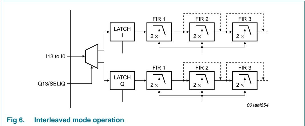
Fig 6. Interleaved mode operation
