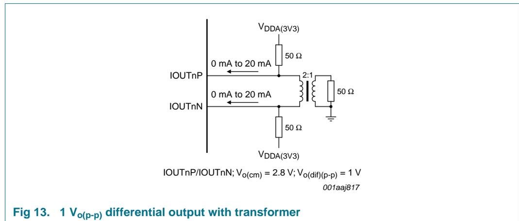
**Fig 13. 1 V<sub>o(p-p)</sub> differential output with transformer**
