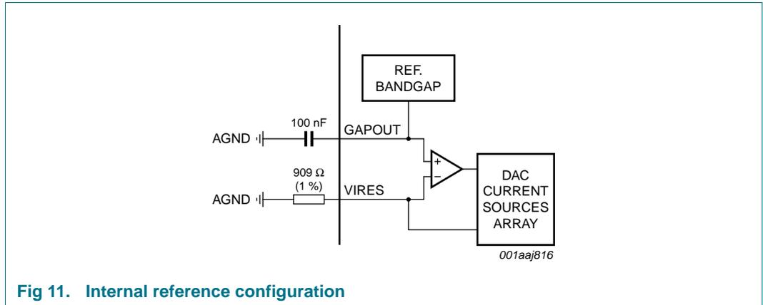
Fig 11. Internal reference configuration
