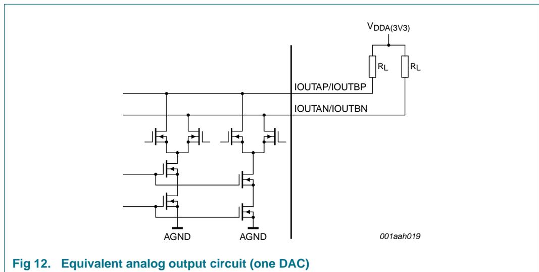
**Fig 12. Equivalent analog output circuit (one DAC)**
