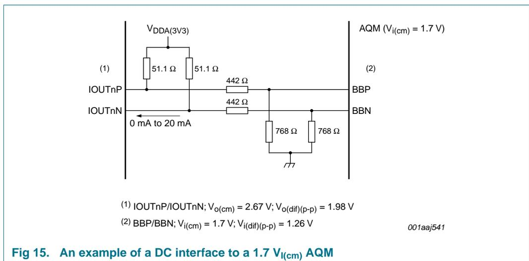
Fig 15. An example of a DC interface to a  $1.7 V_{I(cm)}$  AQM
