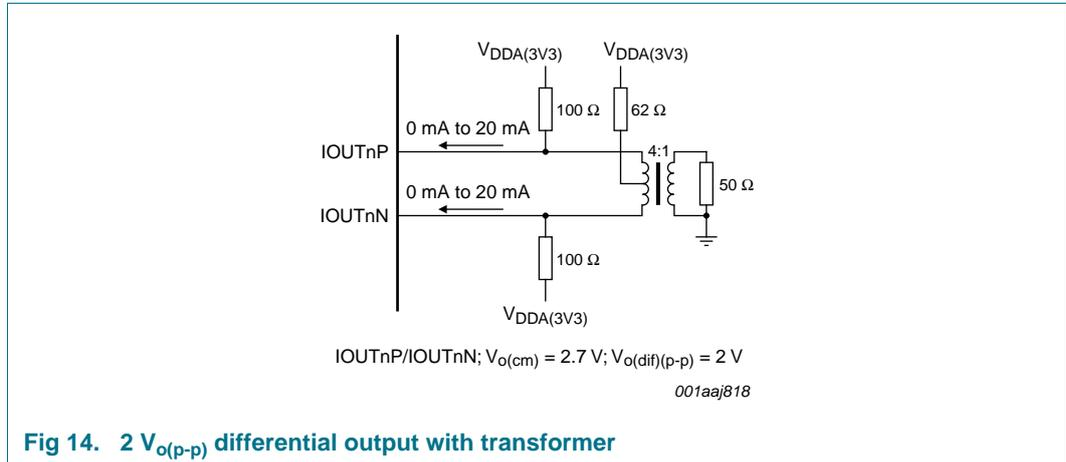
Fig 14.  $2 V_{O(p-p)}$  differential output with transformer
