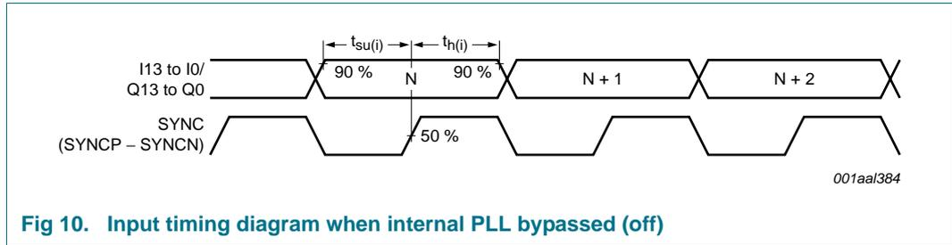
Fig 10. Input timing diagram when internal PLL bypassed (off)
