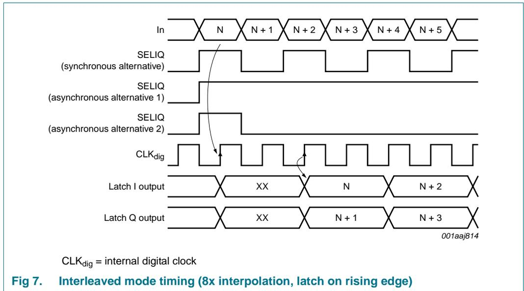
Fig 7. Interleaved mode timing (8x interpolation, latch on rising edge)
