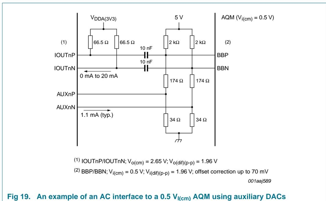
Fig 19. An example of an AC interface to a 0.5  $V_{i(cm)}$  AQM using auxiliary DACs
