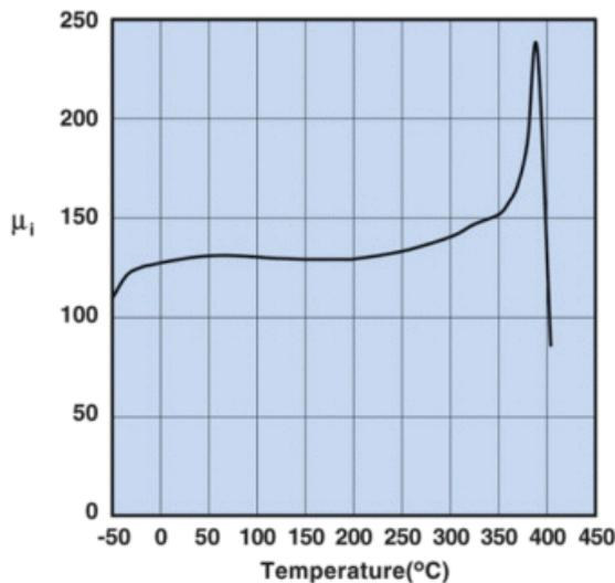
Measured on a 19/10/6mm toroid at 100kHz.
