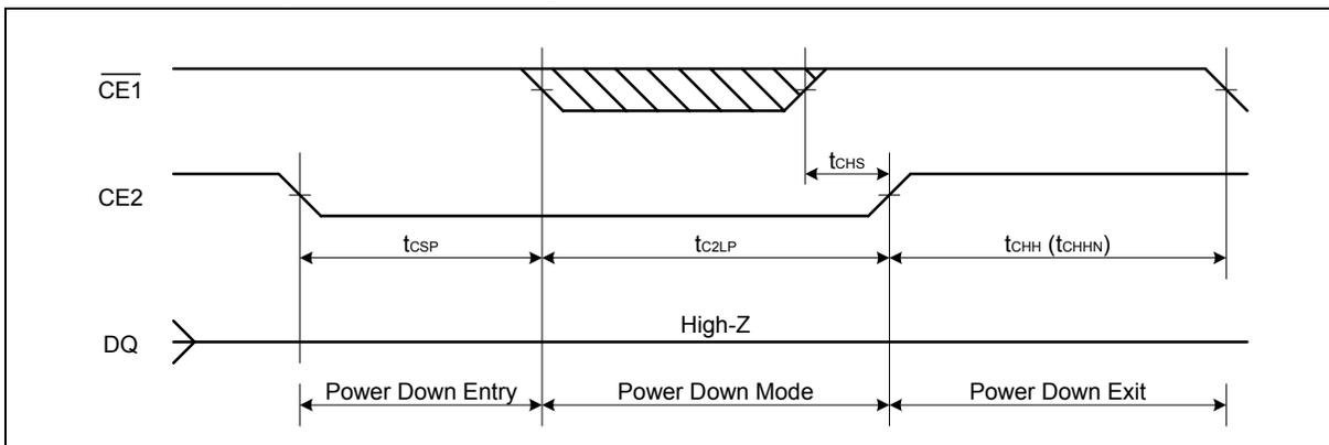
**Note:** This Power Down mode can be also used for Power-up #2 below except that tCHHN can not be used at Power-up timing.
