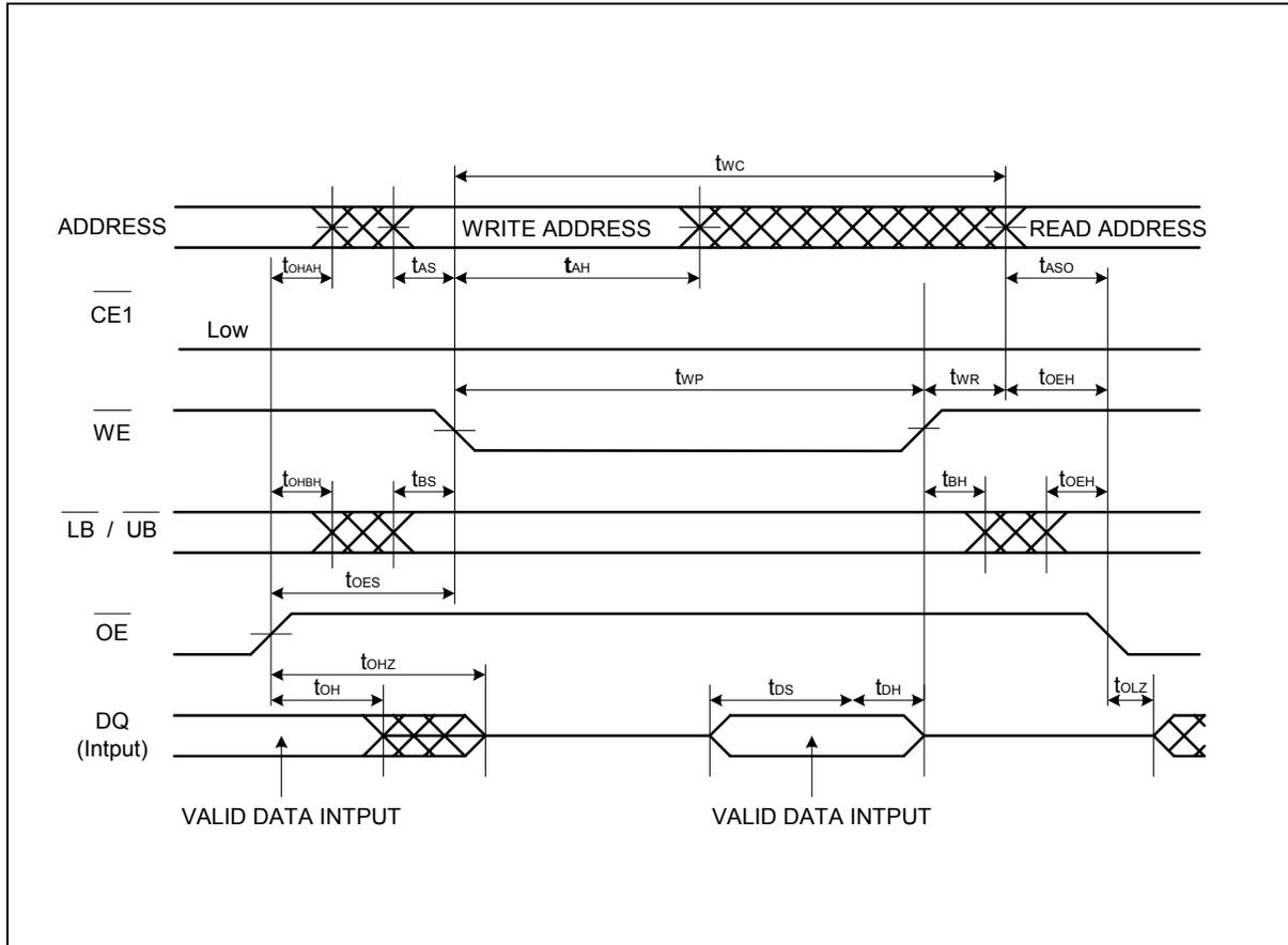
**Note:**  $\overline{\text{CE1}}$  can be tied to Low for  $\overline{\text{WE}}$  and  $\overline{\text{OE}}$  controlled operation.
