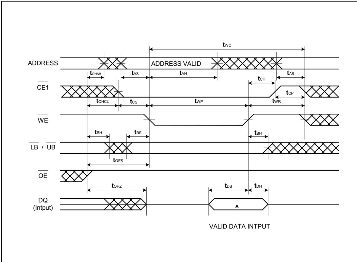
**Note:** CE2 and PE must be High for entire write cycle.
