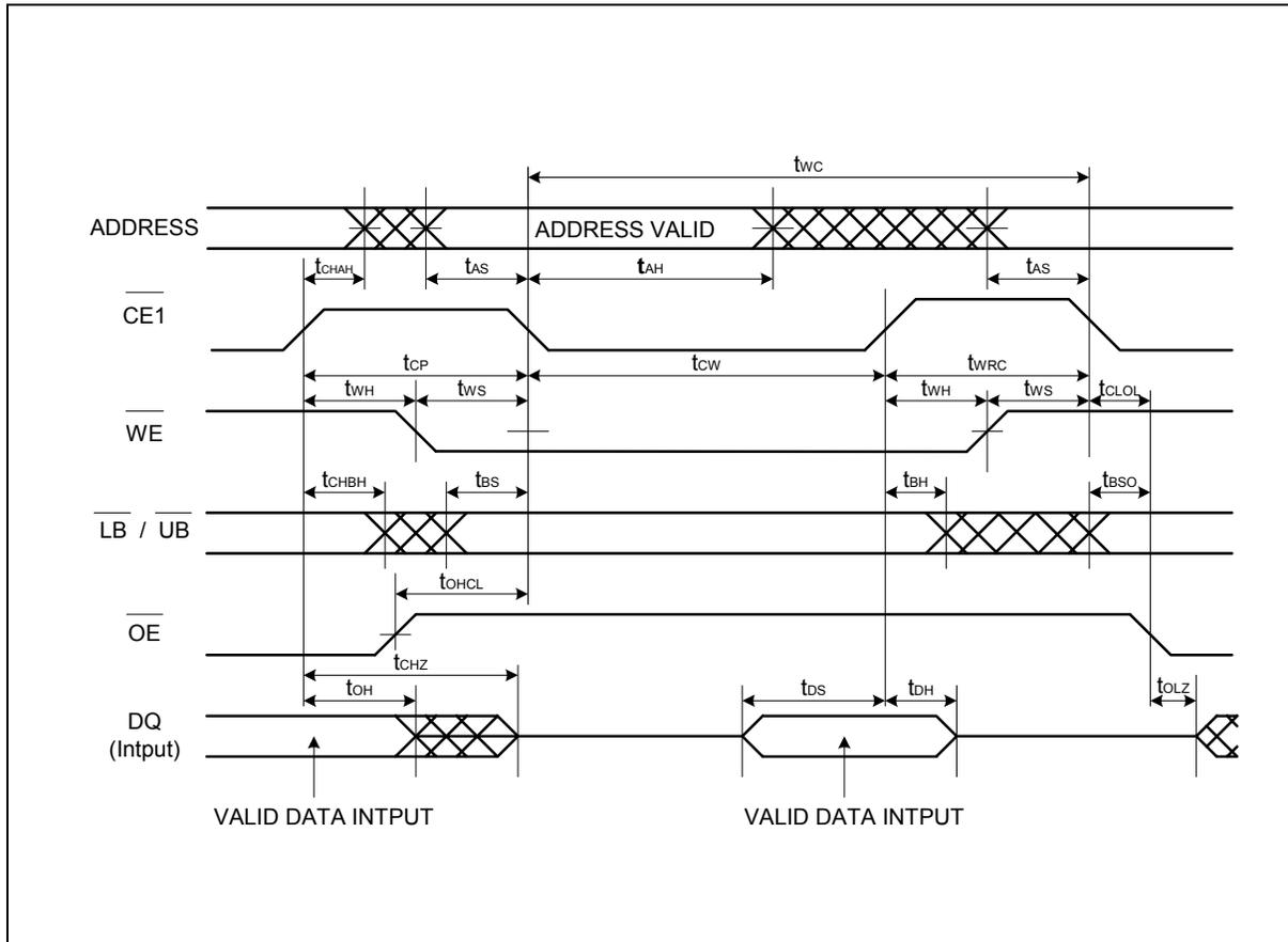
**Note:** Write address is valid from either  $\overline{CE1}$  or  $\overline{WE}$  of last falling edge.
