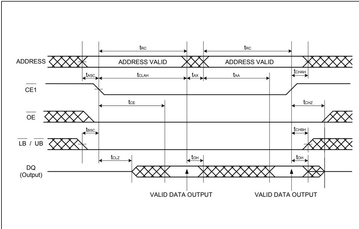
**Note:**  $\overline{\text{CE2}}$ ,  $\overline{\text{PE}}$  and  $\overline{\text{WE}}$  must be High for entire read cycle.
