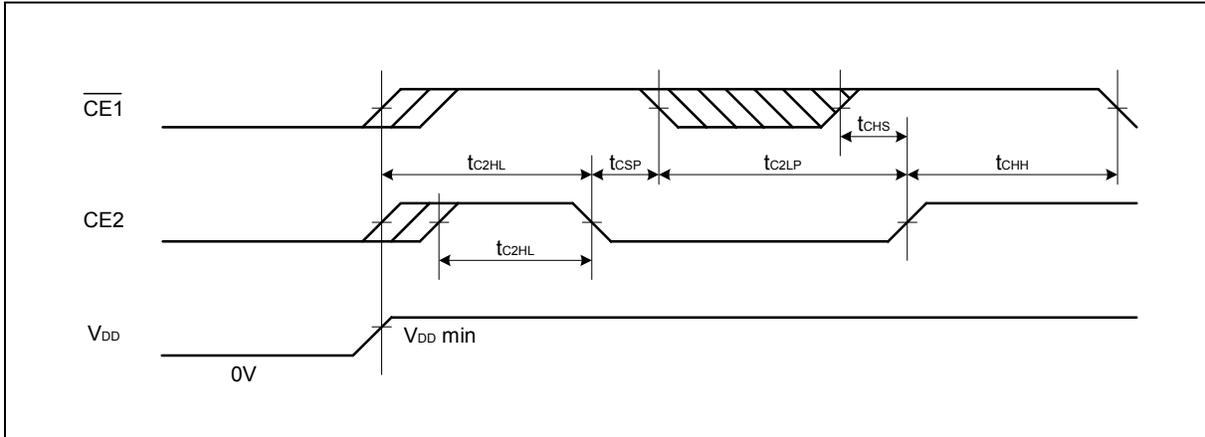
**Note:** The  $t_{c2HL}$  specifies from CE2 low to High transition after  $V_{DD}$  reaches specified minimum level.
