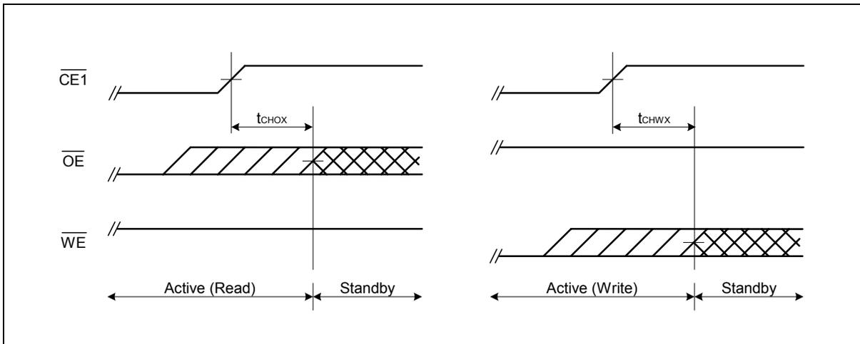
**Note:** Both  $t_{CHOX}$  and  $t_{CHWX}$  define the earliest entry timing for Standby mode. If either of timing is not satisfied, it takes  $t_{RC(min)}$  period from either last address transition of A0, A1 and A2, or  $\overline{CE1}$  Low to High transition.
