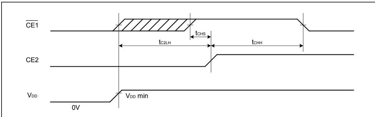
**Note:** The tC2LH specifies after VDD reaches specified minimum level.
