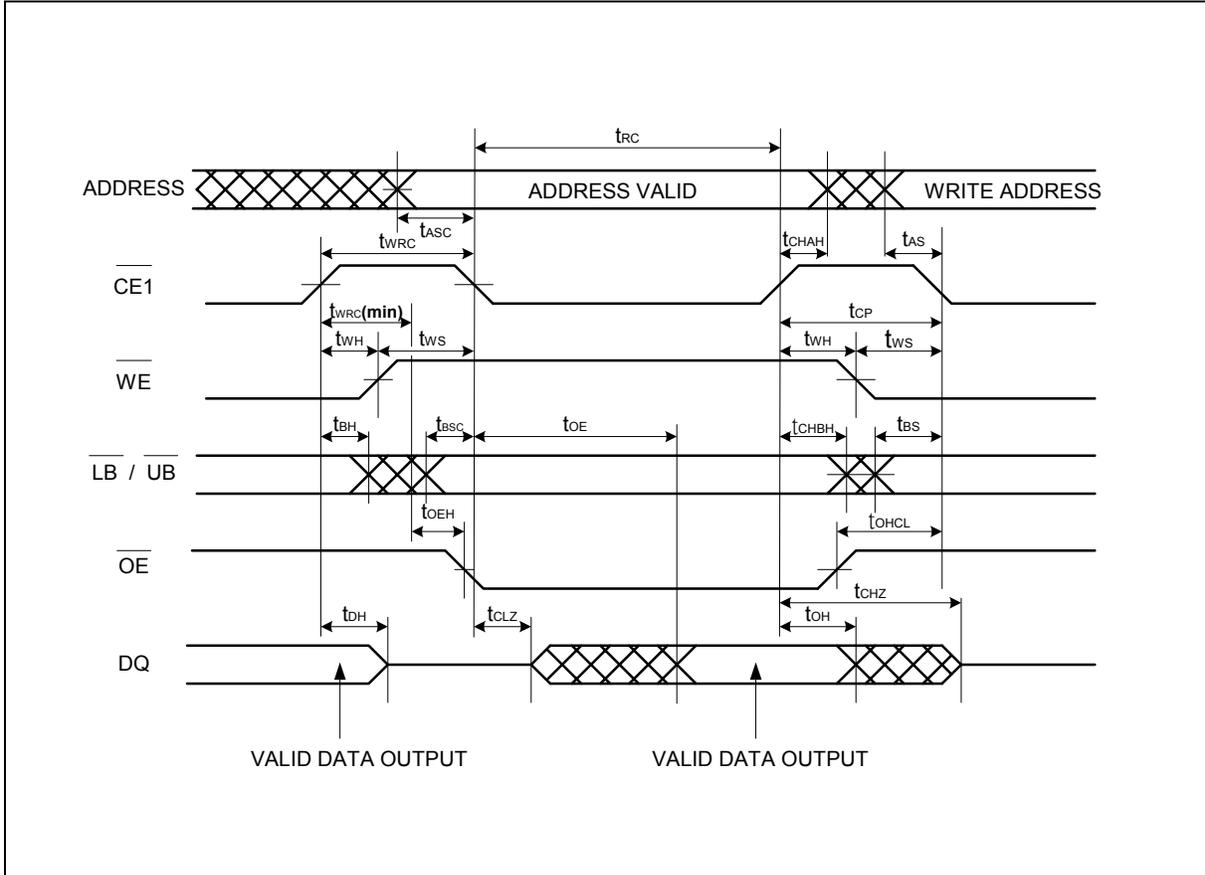
**Note:** The  $t_{OE}$  is specified from the time satisfied both  $t_{WRC}$  and  $t_{WR}(\min)$ .
