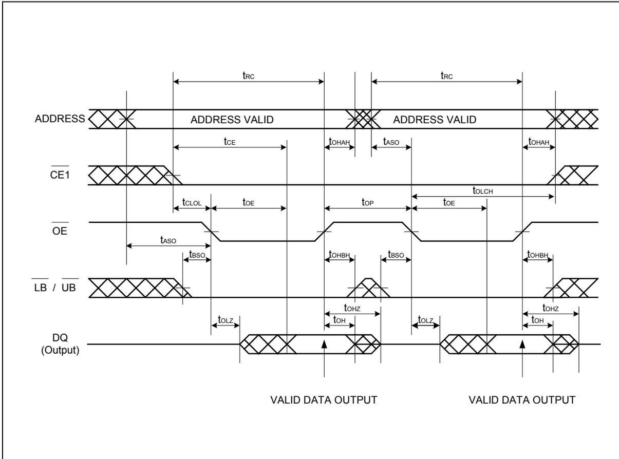
**Note:**  $\overline{CE2}$ ,  $\overline{PE}$  and  $\overline{WE}$  must be High for entire read cycle.
