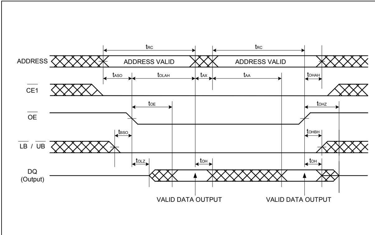
**Note:** CE2,  $\overline{\text{PE}}$  and  $\overline{\text{WE}}$  must be High for entire read cycle.
