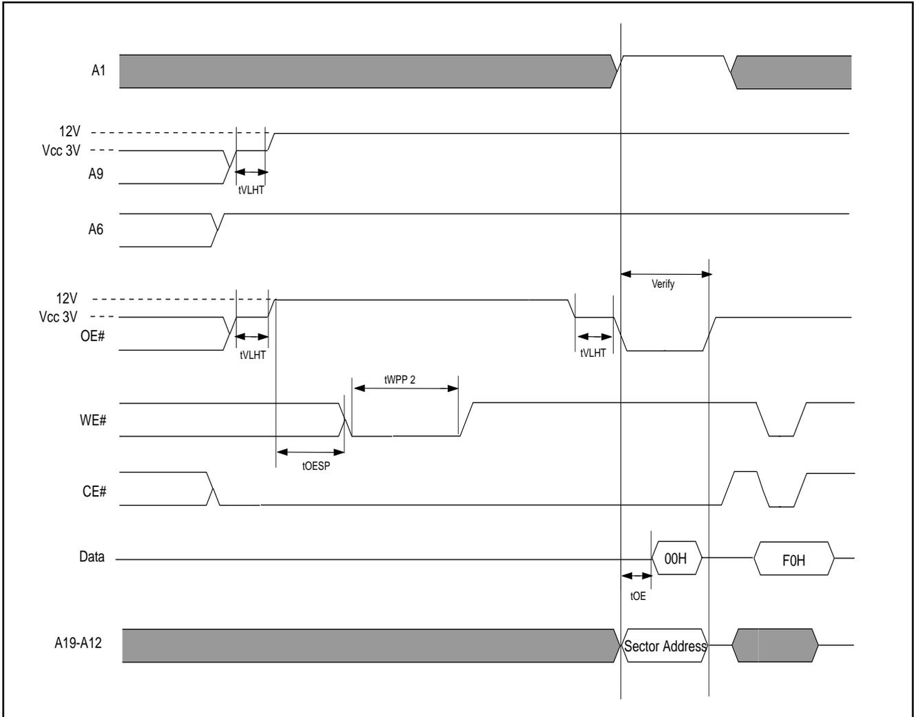
Figure 17. CHIP UNPROTECTION ALGORITHM (A9, OE# Control)
