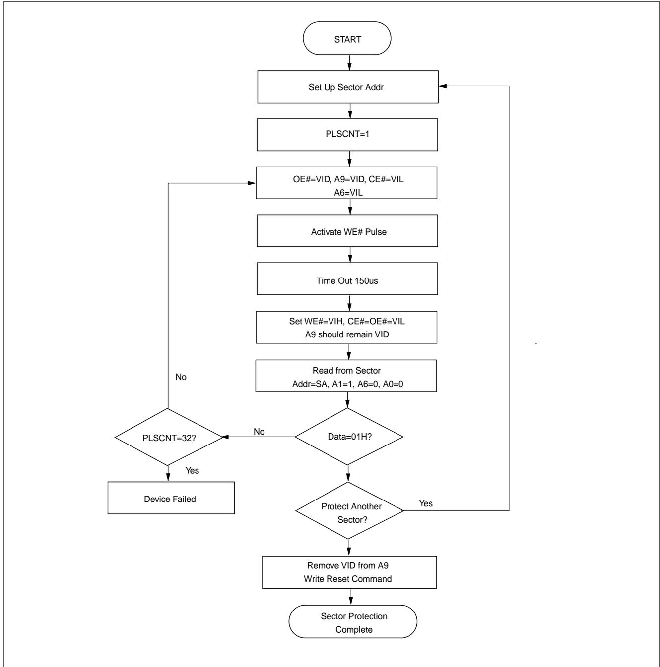
Figure 14. IN-SYSTEM SECTOR PROTECTION ALGORITHM WITH RESET# = VID
