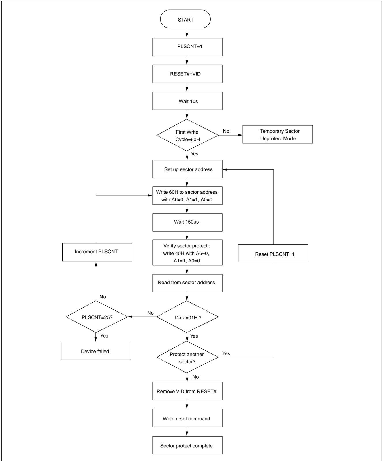
Figure 15. IN-SYSTEM CHIP UNPROTECTION ALGORITHM WITH RESET#=VID
