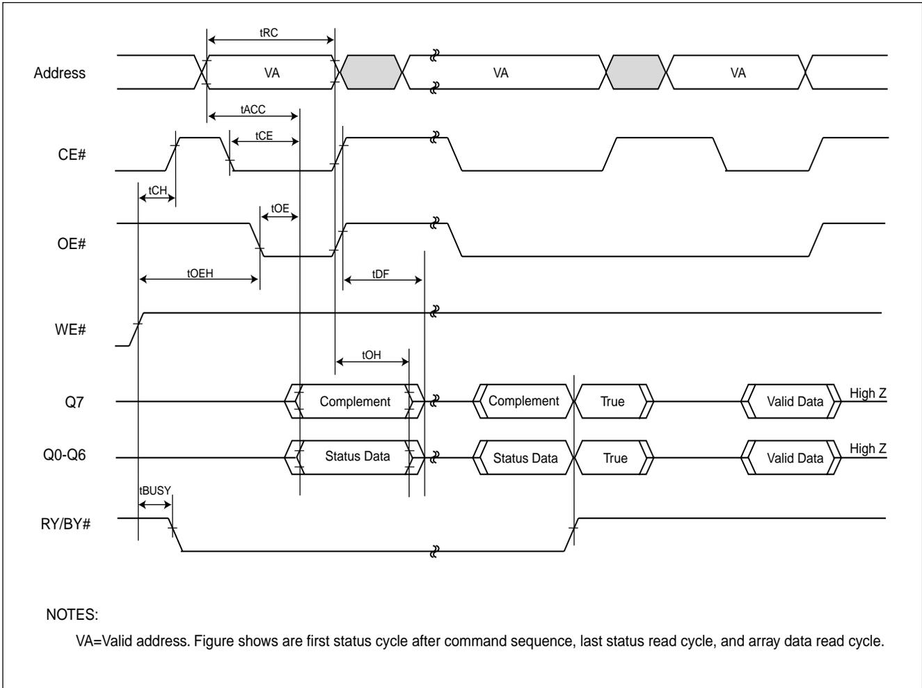
**Figure 21. TOGGLE BIT TIMING WAVEFORMS (DURING AUTOMATIC ALGORITHMS)**
