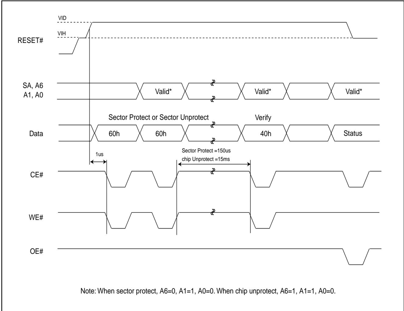
**Figure 12. SECTOR PROTECT TIMING WAVEFORM (A9, OE# Control)**
