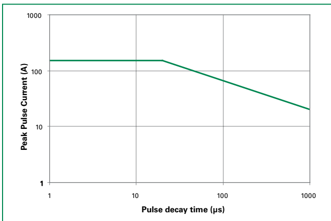
Figure 1: Non-repetitive Peak Pulse Current vs. Pulse Time
