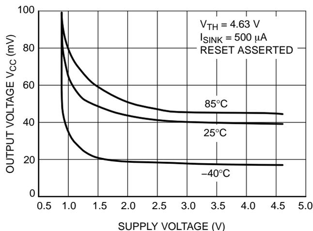
Figure 7. Output Voltage Low vs. Supply Voltage
