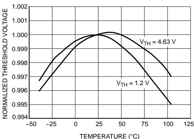
Figure 5. Normalized Reset Threshold Voltage vs. Temperature
