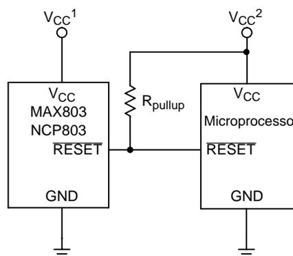
Figure 13. MAX803 RESET Output with Two Supplies
