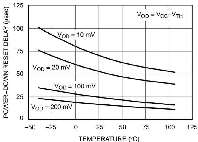
**Figure 8. Power-Down Reset Delay vs. Temperature and Overdrive ( $V_{TH} = 1.2\text{ V}$ )**
