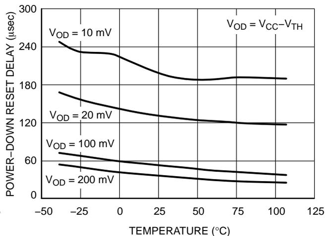
**Figure 9. Power-Down Reset Delay vs. Temperature and Overdrive ( $V_{TH} = 4.63\text{ V}$ )**
