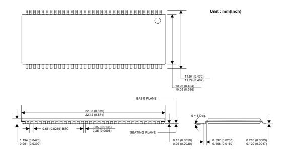
Note: Package do not mold protrusion. Allowable protrusion of both sides is 0.4mm.
