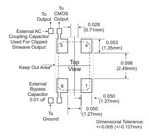
\* Do not route any traces in the keep out area. It is recommended the next layer under the keep out area is to be ground plane.
