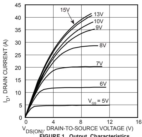
FIGURE 1, Output Characteristics
