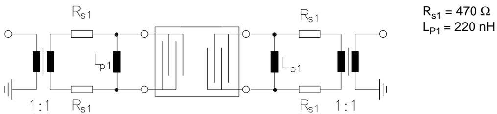
The insertion attenuation of the above mentioned network includes 26,8 dB additional loss due to the impedance transformation to 1000Ω and the losses of the two baluns.
