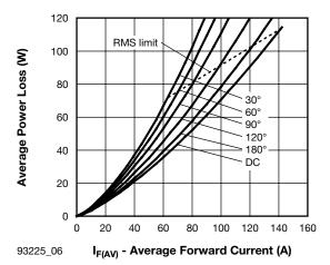
Fig. 6 - Forward Power Loss Characteristics
