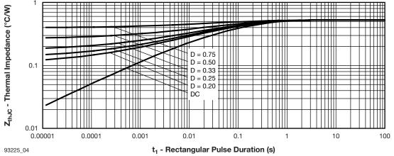
Fig. 4 - Maximum Thermal Impedance Z<sub>thJC</sub> Characteristics
