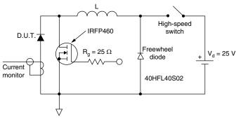
Fig. 8 - Unclamped Inductive Test Circuit
