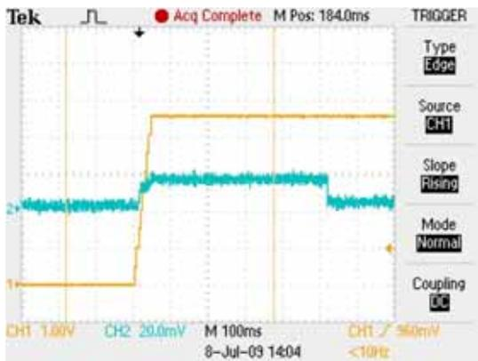
Figure 2: Startup Pop-Noise Reduction with PA4220 (32 Ω load)
