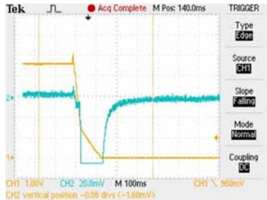
Figure 3: Shutdown Noise without PA4220 (32 Ω load)
