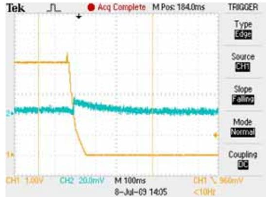
Figure 4: Shutdown Noise with PA4220 (32 Ω load)
