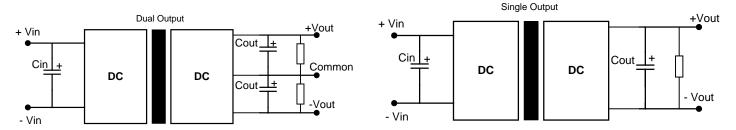
All the AM3LV-Z Series have been tested with the above recommended test circuit. This series should be tested under load.
