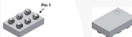
Figure 1. WLCSP Bump Configuration (Top & Bottom)
