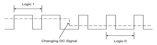
\*Only 50/50 duty cycle data is suitable for the T433 transmitter and R433 receiver.
