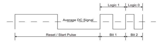
A 50/50-duty cycle will have an average DC signal resulting in a constant reference for the data slicer. Users should use pulse-width modulation to transmit data with logic 1's or 0's.
