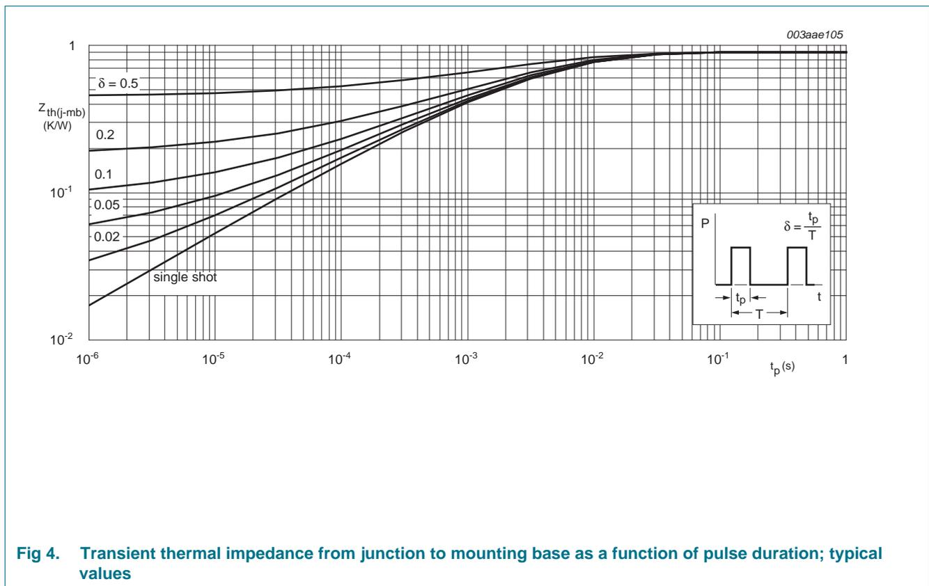
Fig 4. Transient thermal impedance from junction to mounting base as a function of pulse duration; typical values
