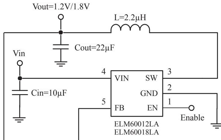
\* Passive components without specified values in the above figure are optional.
