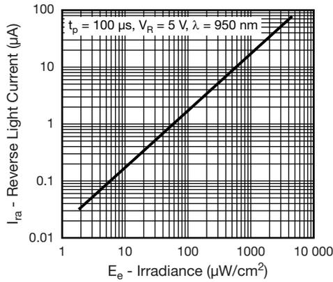
Fig. 3 - Reverse Light Current vs. Irradiance
