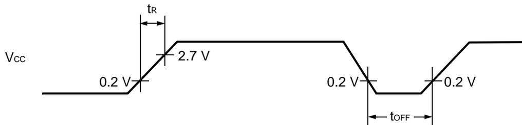
Sudden changes in the power supply voltage may cause a power-on reset. To change the power supply voltage while the device is in operation, it is recommended to raise the voltage smoothly to suppress fluctuations as shown below. In this case, change the supply voltage with the PLL clock not used. If the voltage drop is 1 V or fewer per second, however, you can use the PLL clock.
