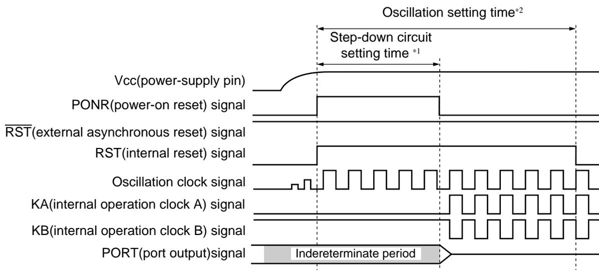
\* : 1: Step-down circuit setting time :  $2^{17}$ /oscillation clock frequency (oscillation clock frequency of 16 MHz: 8.19 ms)
