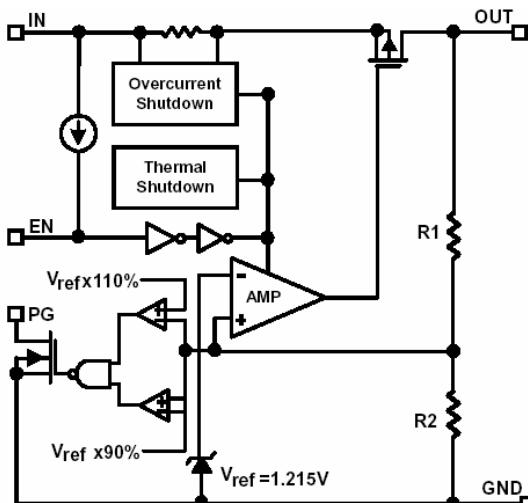
Note: If output voltage specification is lower than 1.215V, Vref will be trimmed to 1.2V
