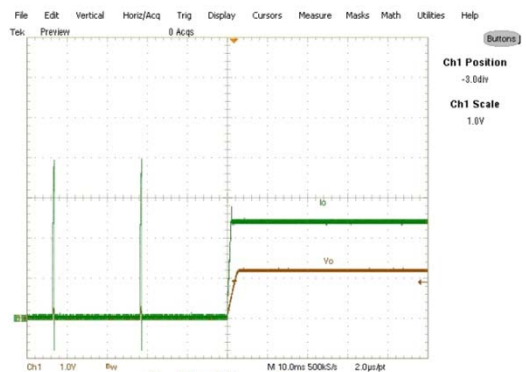
Fig. 12: Short circuit (Hiccup) Recovery Ch 1 :V out , Ch 4 :Iout
