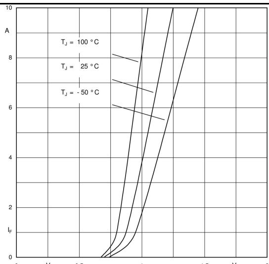
Fig. 1 Forward characteristics (typical values)
