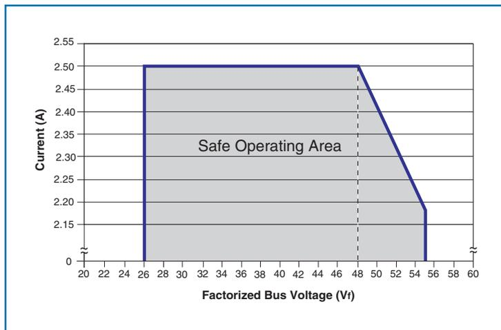
**Figure 17** — PR024A480T012FP rating based on Factorized Bus voltage
