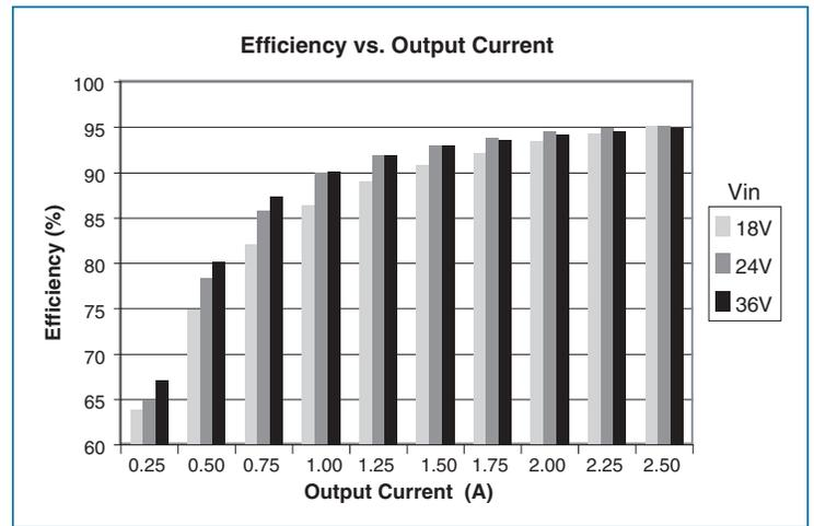
Figure 6 — Efficiency vs. output current at 36 Vf
