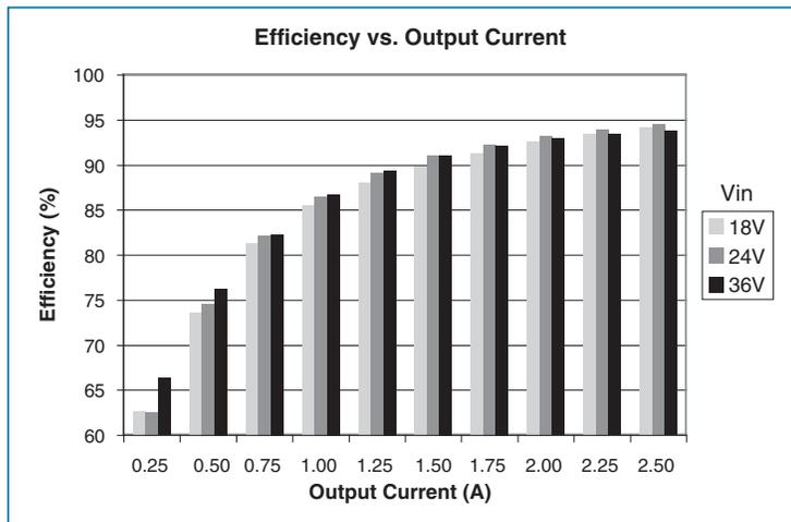
Figure 7 — Efficiency vs. output current at 26 Vf
