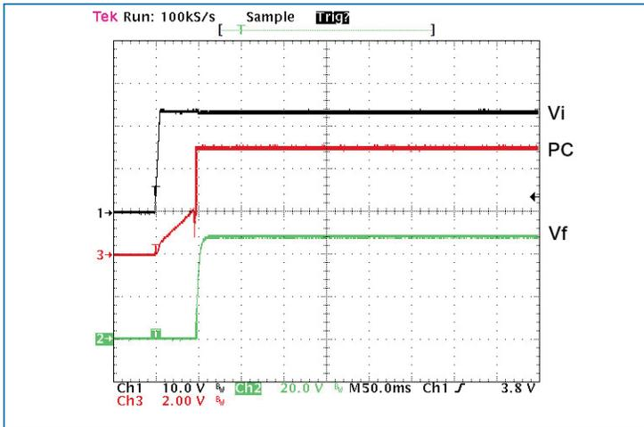
Figure 1 — Vf and PC response from power up
