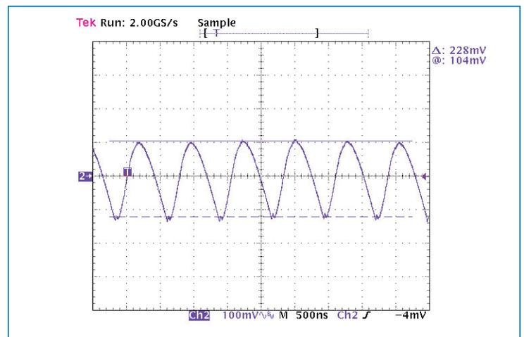
**Figure 13** — Output ripple full load 10 µF bypass capacitance
