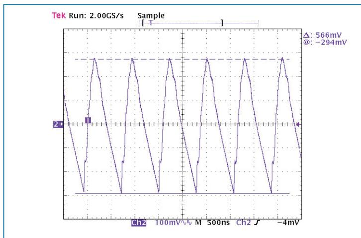
**Figure 12** — Output ripple full load no bypass capacitance
