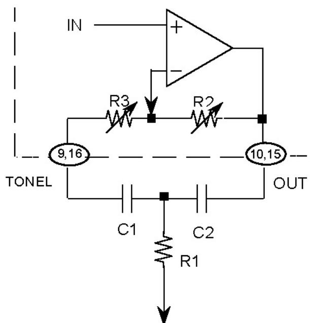
$$F_0 = \frac{1}{2\pi\sqrt{R_1(R_2+R_3)C_1C_2}} \text{ (Hz)}$$
