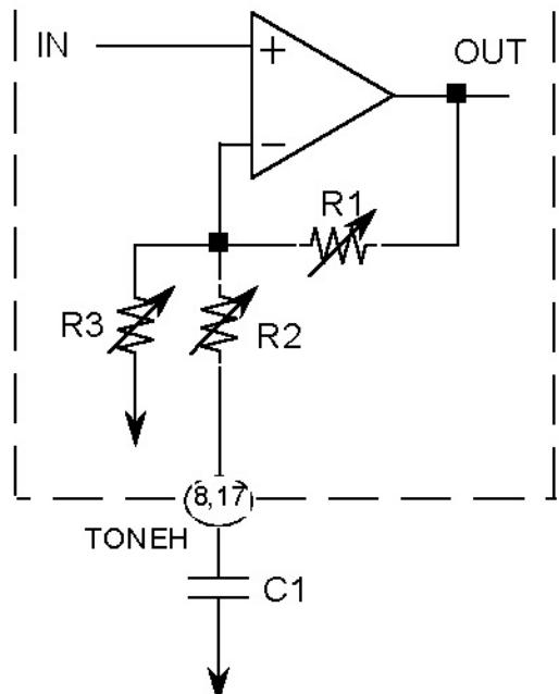
$$F_c = \frac{1}{2\pi \cdot R_2 \cdot C_1} \text{ (Hz)}$$
