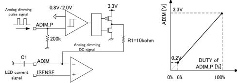
Figure 12. Analog dimming function and character
