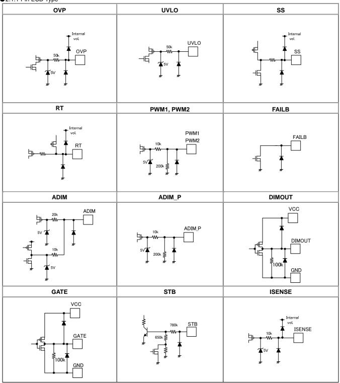
Figure 4-1. Internal equivalent circuit
