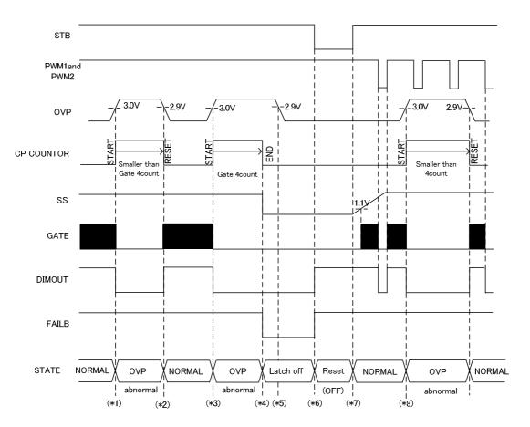
(\*1)...As OVP is detected, the output GATE=L, DIMOUT=L, and the CP counter starts
