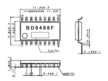
Figure 3-1. Pin configuration
