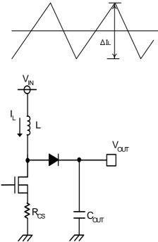
The inductor value affects the input ripple current. The equality in the section 3.5.1 is as following.
