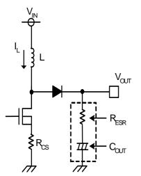
Output capacitor needs to be selected in consideration of equivalent series resistance required to even the stable area of output voltage or ripple voltage. Be aware that set LED current may not be flown due to decrease in LED terminal voltage if output ripple componet is high. Output ripple voltage  $\Delta V_{OUT}$  is determined by Equation (4):
