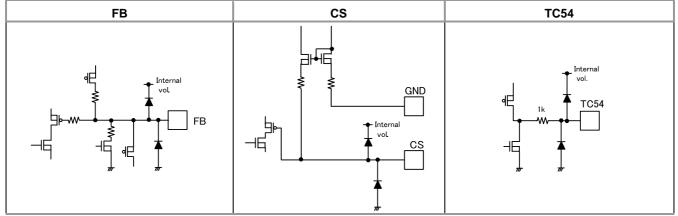
Figure 4-2. Internal equivalent circuit
