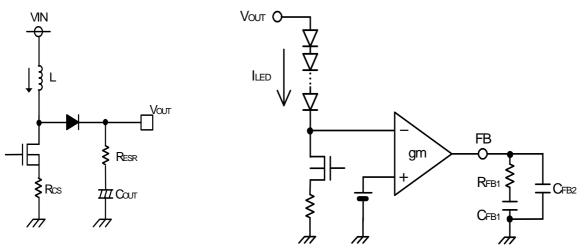
Figure 31. the circuit of output stage and the error amplifier
