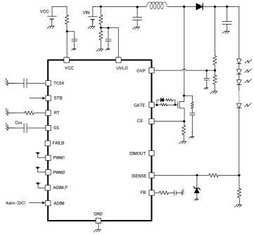
Figure 19. the circuit example of analog dimming only
