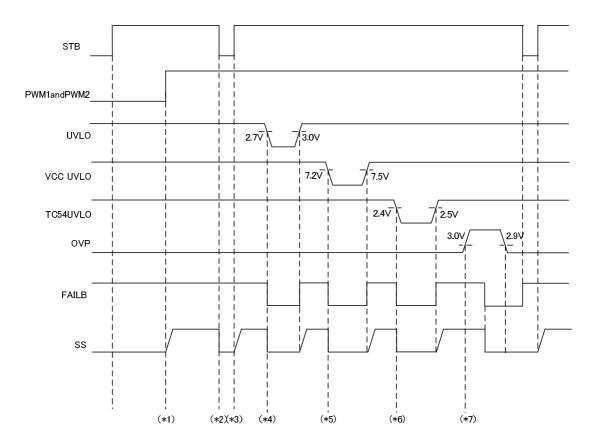
(\*1)...The SS pin charge does not start by just STB=H. "PWM1=H and PWM2=H" is required to start the soft start. In the low SS voltage, the GATE pin duty is depend on the SS voltage. And as the SS is less than 1.1V, the pulse does not output. (\*2)...By the low STB=L, the SS pin is discharged immediately.
