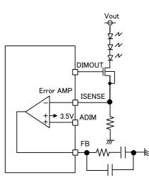
Figure 14. ISENSE pin circuit
