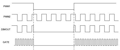
Figure 11. PWM pin function
