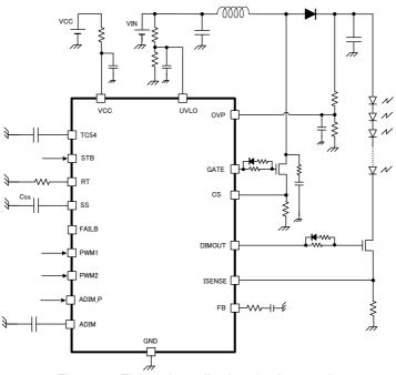
Figure 16. The basic application circuit example
