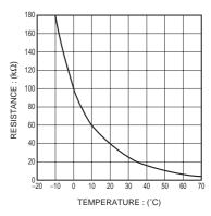
Fig.5 Thermistor curve
