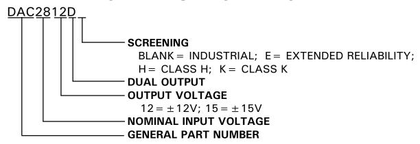
The above example is an industrial grade  $\pm 12V$  dual output converter
