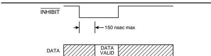
FIGURE 18. INHIBIT TIMING
