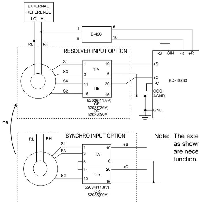
Note: The external BW components as shown in Figures 1 and 2 are necessary for the R/D to function.
