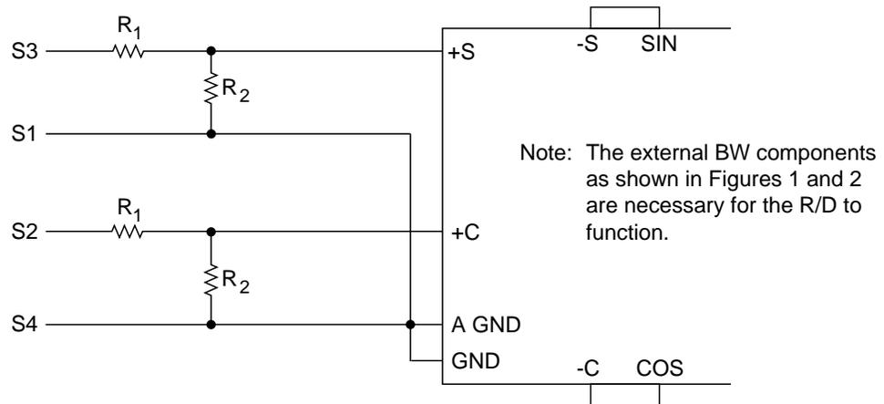
$$\frac{R_2}{R_1 + R_2} = \frac{2}{X \text{ Volt}}$$
