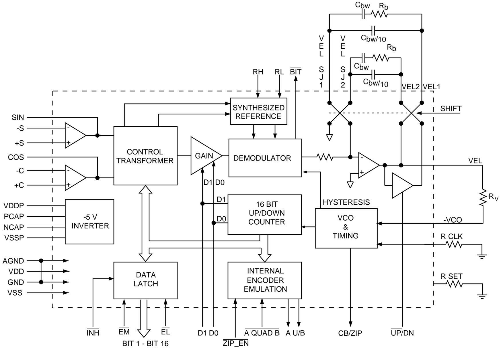
FIGURE 1. RD-19230 SERIES BLOCK DIAGRAM
