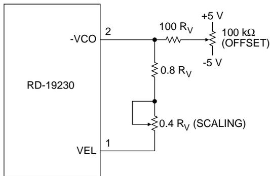
FIGURE 15. VELOCITY TRIMMING
