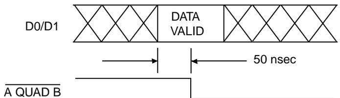
**FIGURE 23. TIMING FOR INCREMENTAL ENCODER EMULATION RESOLUTION CONTROL**
