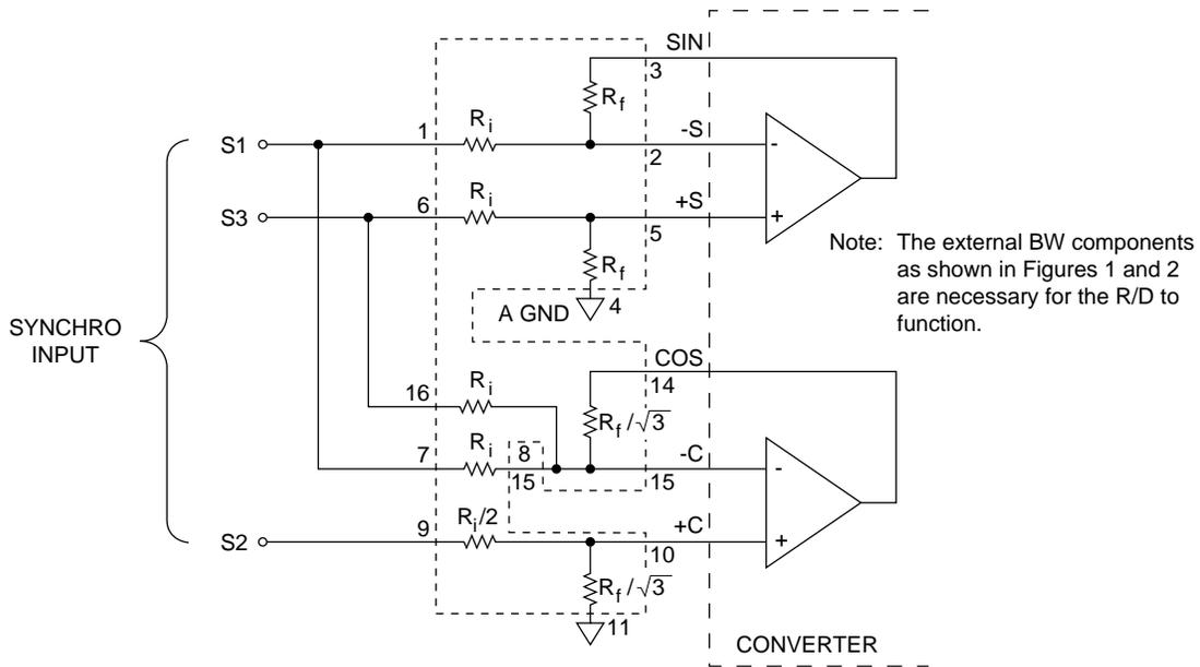
S1, S2, S3 should be triple twisted shielded; RH and RL should be twisted shielded;
