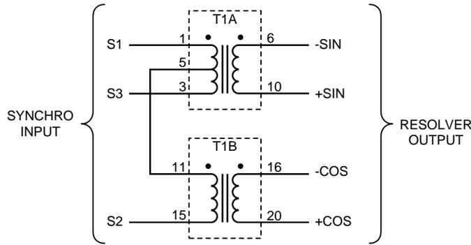
**FIGURE 6. TRANSFORMER LAYOUT AND SCHEMATIC (SYNCHRO INPUT - 52034/52035)**
