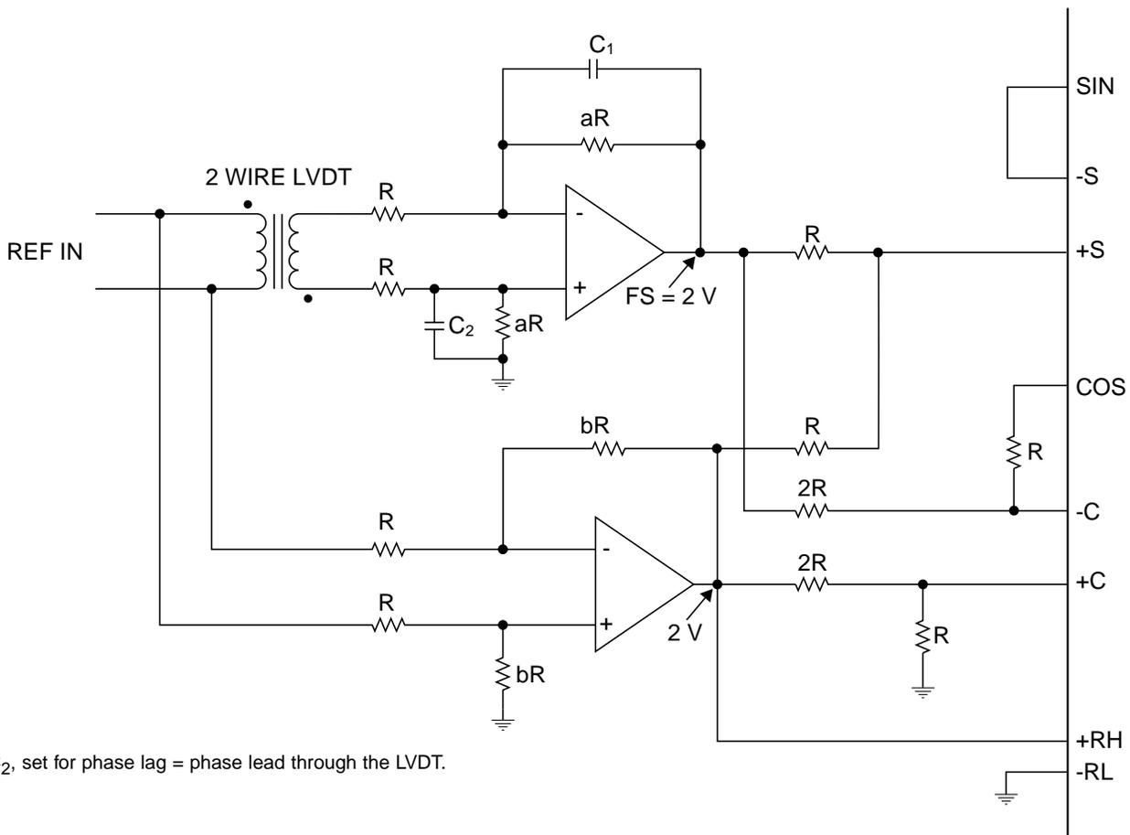
$C_1 = C_2$ , set for phase lag = phase lead through the LVDT.
