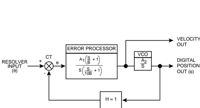
FIGURE 3. TRANSFER FUNCTION BLOCK DIAGRAM #2
