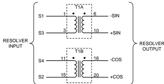
**FIGURE 7. TRANSFORMER LAYOUT AND SCHEMATIC (RESOLVER INPUT - 52036/52037/52038)**
