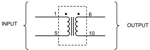
**FIGURE 8. TRANSFORMER LAYOUT AND SCHEMATIC (REFERENCE INPUT - B-426)**
