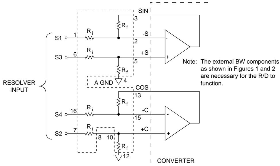
S1 and S3, S2 and S4, and RH and RL should be ideally twisted shielded, with the shield tied to GND at the converter.
