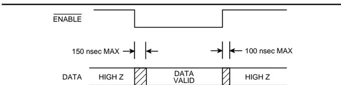
FIGURE 19. ENABLE TIMING
