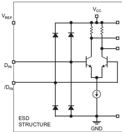
Figure 2. Input Structure
