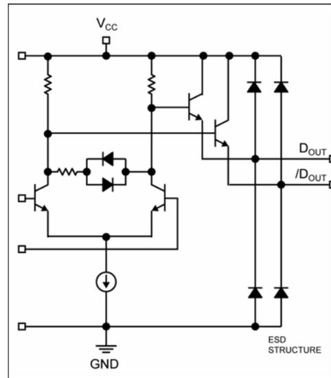
Figure 3. Output Structure
