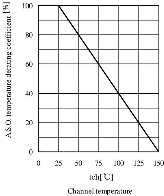
MOSFET A.S.O Curve  $T_a = 25^\circ\text{C}$
