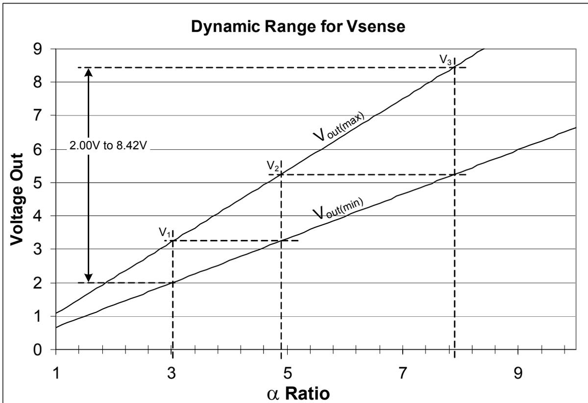
Figure 6. Graphical Determination of the  $\alpha$  Ratios
