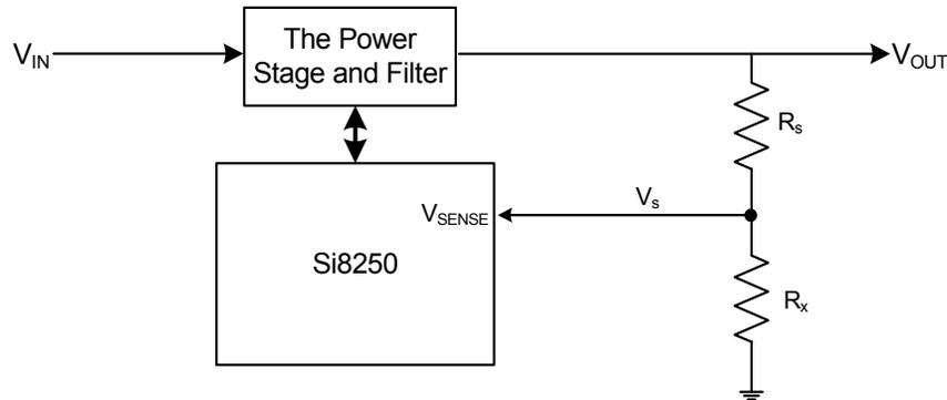
**Figure 3. Resistor Divider**
